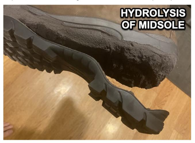
Hydrolysis is a double decomposition reaction, with water as one of the reactants. Simply put, the oxygen atom in water bonds with the carbon atom of the polyesters in the Polyurethane. This carbon-oxygen bond is unstable, and eventually also breaks down, leading to the gradual disintegration of the polyester Polyurethane.
